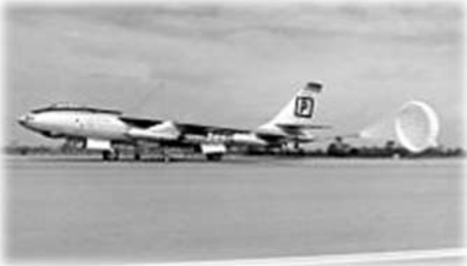
Boeing B-47B-40BW of the 306th Bomb Wing (Medium) at MacDill AFB, Florida, landing with drag chute.
