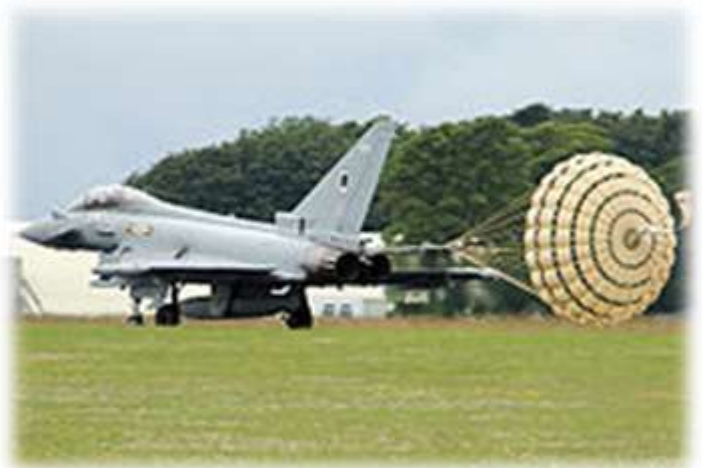
RAF Typhoon using a parachute for braking after landing
