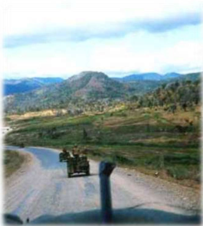
A 404th RRD (Abn) convoy in the vicinity of Mang Yang Pass, Route 19. Object lower center on hood of vehicle is fabricated to cut garrote wires strung across roads by the enemy.
